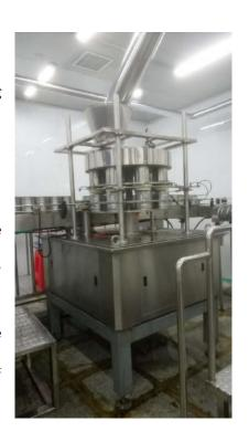
requirements of food hygiene. This equipment is driven by variable frequency speed regulating motor, and the production capacity is graded and adjustable.
