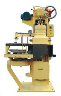
the tank and the lid hook in good bending hook, the second seal wheel is after the first joint after the formation of the seal. The symmetrical head channel and two channel structures make the sealing quality of the large tank more stable. With a vacuum system, it can vacuum the tank, no longer equipped with a steam exhaust box, reducing the cost of the product, and extending the shelf life of the can.
