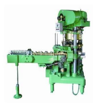
cannery and beverage factory. This machine uses steam to meet the vacuum requirements in the tank.
